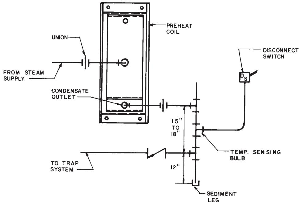
Temperature sensing bulb is located in Tee. Disconnect switch is used to control blower motor and close fresh air damper when condensate temperature drops below any set temperature between 45° and 60°F.
